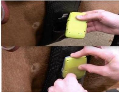
Figure 1: Placement of the equinITY™ heart rate monitoring system and girth.
